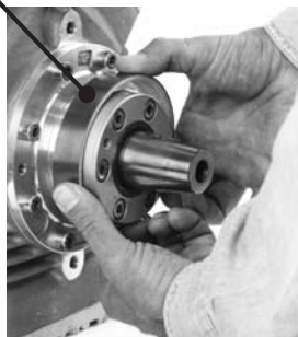
Leak oil collection ring
